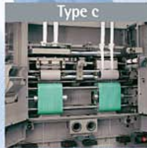
Short drafting system with control barrels on wide apron
